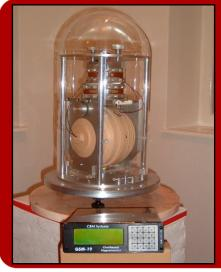
The dldD Suspended System Vector Magnetometer utilizes GEM Systems Overhauser or Potassium sensor technology and provides enhanced precise measurements for the Earth's
