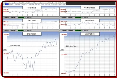
The dIdD data output includes; Total Field, Vertical, North and East (Z, X, Y) component fields as well as changes to the calculated declination and inclination of the Magnetic Field. The dldD system is designed to measure very subtle changes in the Earth's Field.
